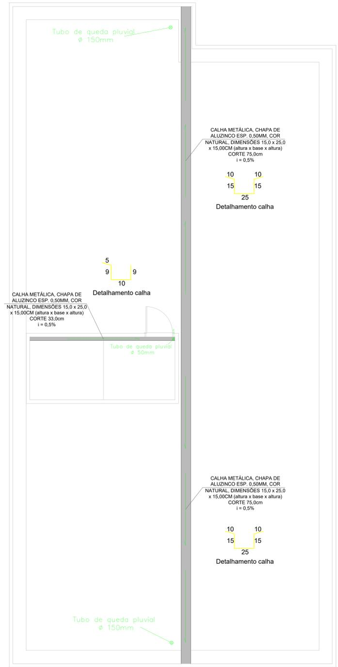
CALHA METÁLICA, CHAPA DE ALUZINCO ESP. 0,50MM, COR NATURAL, DIMENSÕES 15,0 x 25,0 x 15,00CM (altura x base x altura) CORTE 75,0cm
